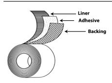
**Backing:** Woven Polyethylene (Printed)
