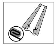
2. Bend seam up to 90° on brake as indicated in drawing.
