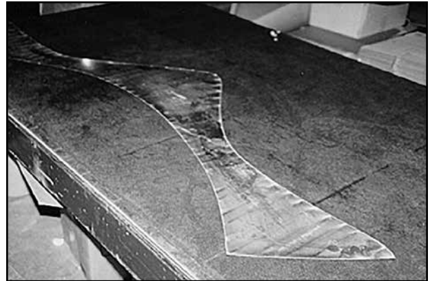
Figure 9-17. Flat pattern on bench
