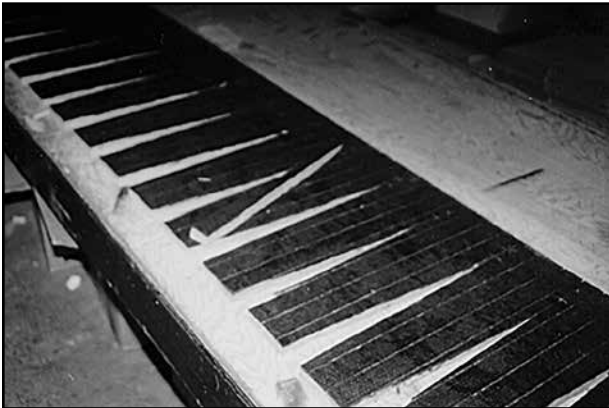
Figure 9-3. Liner board on bench with vee notches
