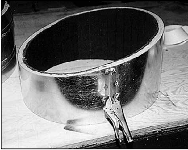
Figure 7-6. Finished gore insulation section
