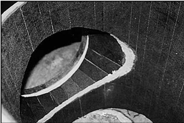
Figure 9-14. Inside view of tapered tap
