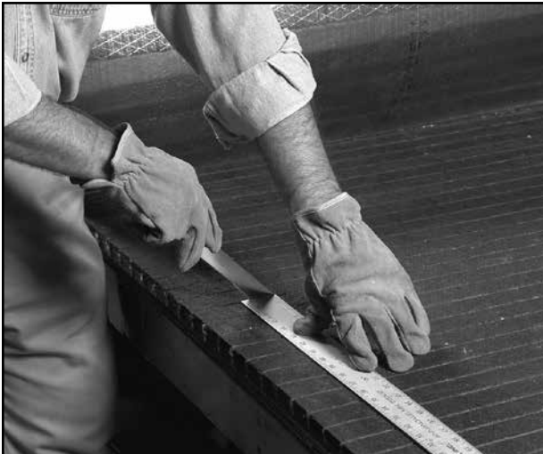
Figure 5-14. Measuring for stretchout
