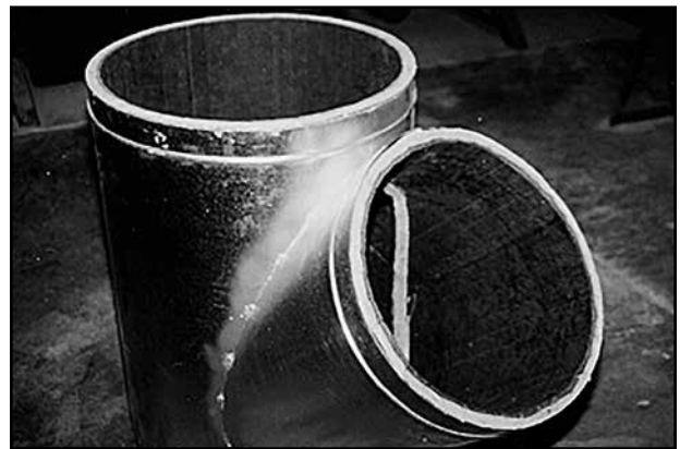
Figure 9-1. Angled tap on straight-through body
