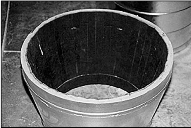
Figure 8-7. Taper insert in duct
