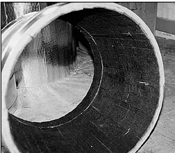
Figure 8-8. Finished taper section
