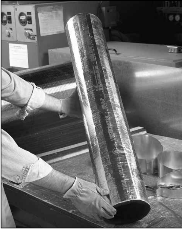
Figure 5-20. Completed insulation section with longitudinal seam taped
