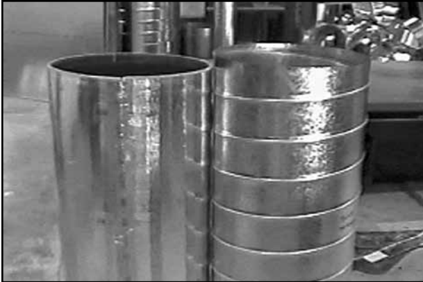
Figure 5-6. Formed liner and spiral duct
