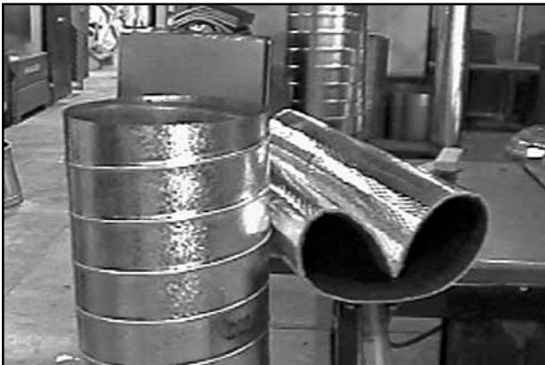
Figure 5-7. Liner folded inward
