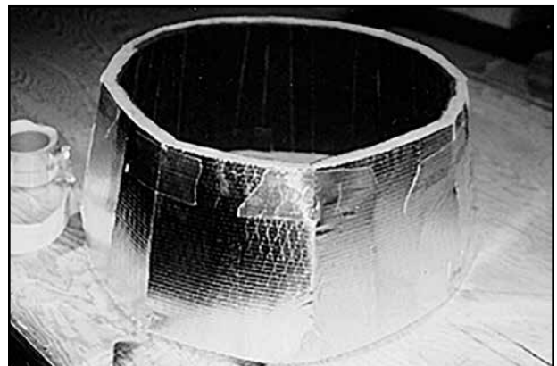
Figure 8-6. Taper insert with wedge cuts closed
