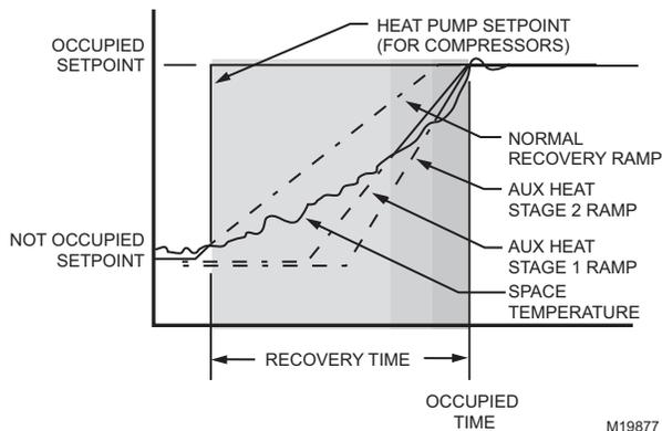
Fig. 11. Heat Setpoint Ramping for Heat Pump Systems.
