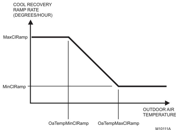
Fig. 12. Setpoint Ramping Parameters with Ramp Rate Calculation.
