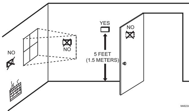
**Fig. 2. Typical Location of Thermostat or Remote-Mounted Sensor.**
