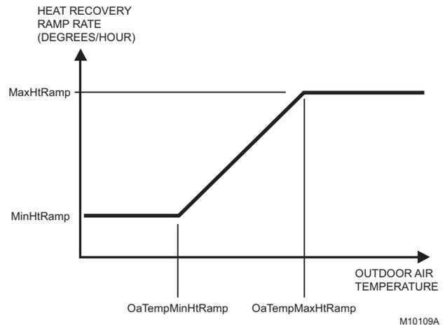
Fig. 10. Heat Setpoint Ramping for Conventional Systems.
