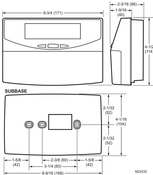
Fig. 1. Thermostat and Subbase Dimensions in inches (mm).
