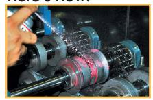
1. Spray The Stripper at those points where galvanizing tends to build up on your machines. The special cleaning ingredients get right to work softening up deposits.
