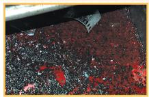
2. Under normal conditions, galvanizing build-up will loosen and flake off by itself after being sprayed with The Stripper. Then if required, remaining build-up can easily be removed by liaht scrapina.
