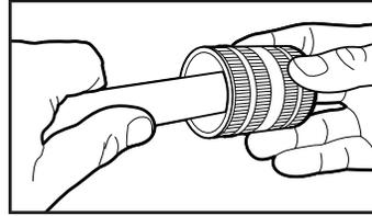
**2** Deburr tube ID & OD using a deburring tool. Ensure tube ends are free of any burrs or sharp edges.
