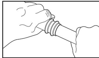
**6** Slightly rotate the fitting while sliding it onto tube. Slide all the way to insertion mark & make contact with stop.
