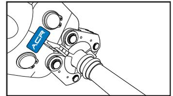
**7b** For 1-1/8", use the Streamline® ACR Press Ring, Ring Jaw, and compatible full-sized press tool. Place Press Ring over both beads at right angle to tube. Use ring jaw to start the pressing process.
