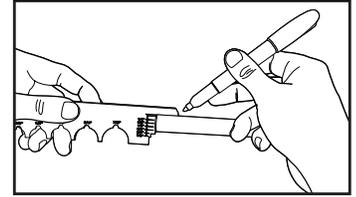
**4** Mark tube to proper fitting insertion depth with the Streamline® ACR Press Gauge or use the insertion depth chart below.
