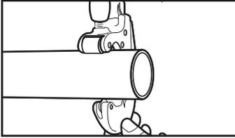
**1** Cut tube square using a tube cutter or fine tooth saw.
