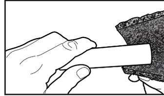
**3** Clean and smooth tube surface using abrasive pad. Tube surface should be free of indentation, scratches and deformations.
