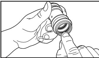
**5** Check both fitting beads to ensure two seals per cup are present.
