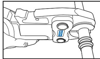
**7a** Place press jaw over both beads at a right angle to the tube. Start the pressing process. See tool manufacturer for tool instruction.
