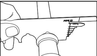
**8** Verify connection is secure using the Streamline® ACR Press Gauge between o-ring beads. Rotate gauge to avoid interference with flashing.
