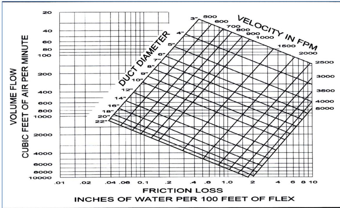
Friction Loss Slide Chart Calculators are available at a minimum cost
